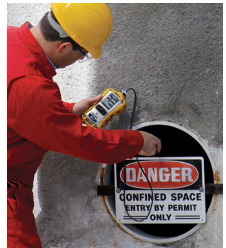
Confined space testing with the MultiRAE Lite
