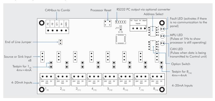
The Combi detects the address being used on this card when connected to the CANbus. This can be checked in engineers menu 27 setup network, the address should be set using the address select switch 220–230.
