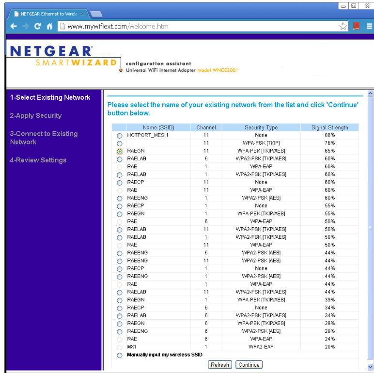
Figure 4. Select a wireless network. (This example shows all available wireless networks within range. Your choices will be different.)
