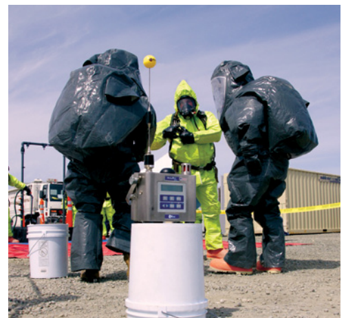
A HazMat Team utilizes the strategically-placed AreaRAE to provide real-time detector to establish a perimeter and monitor PID, LEL and VOC readings.
